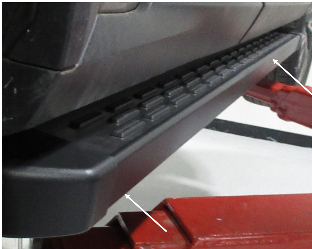
Foto: Trittbrett ohne Metallapplikation Photo: running board (side step) without metal application
