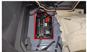
3. Deactivation of high voltage system, use class 0 insulating rubber gloves when operating this disconnect switch.
